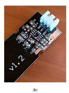
**Figure 5.** (a) Older and (b) recent soil moisture sensor v.1.2. The thin metal path to grounded capacitor plate is clearly visible only in (b).
